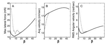
Fig. 6. The effect of  $\beta$  on the recovery from a lateral perturbation with impulse on the order of 2mN-sec. (a) Lateral force (b) Average climbing velocity. (c) Angular velocity. In each plot the solid line is the steady-state behavior (before impulse) and the dotted line is the state 1.5 seconds after impulse.
