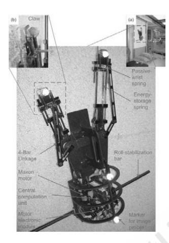
Fig. 9. Picture of the robot with annotations.
