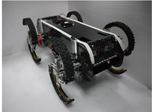
Fig. 1. Photo of the *TurboQuad* robot.
