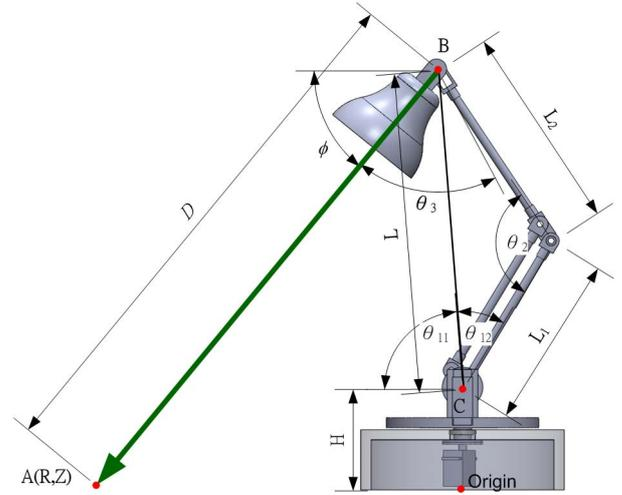
Fig. 5. Symbols for joint angle computation of Disco Lamp.
