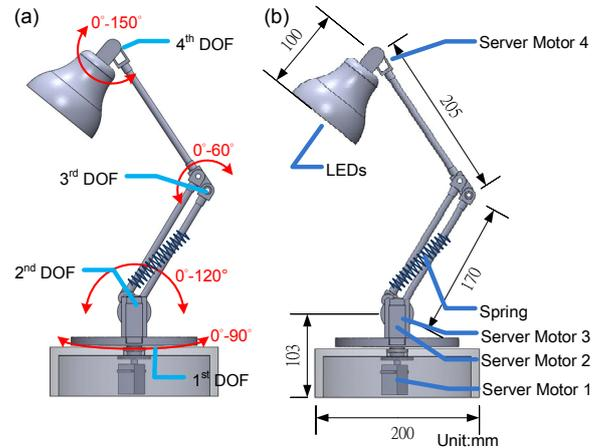
Fig. 2. Mechanism and dimensions of Disco Lamp.
