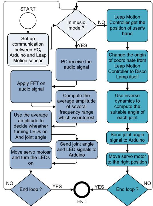
Fig. 4. Program flow chart of Disco Lamp.
