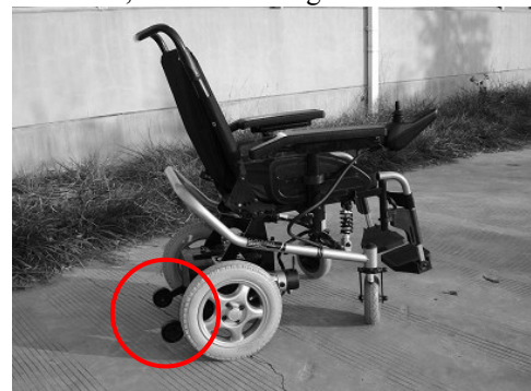
Fig. 1. A wheelchair with an accident-proof device (circled) to prevent overturning [5].
